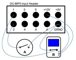
The picture above shows both trigger switches in their 'off' (untriggered) position.
